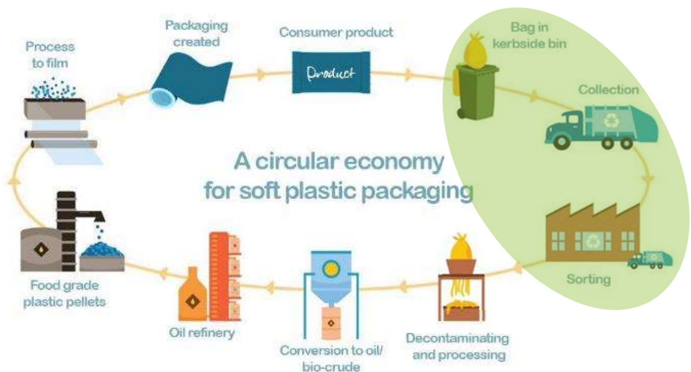
Figure 1 Material flow for the National Plastics Recycling Scheme (trial elements highlighted in green)
